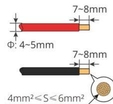
Step 2: Assembling the Crimp contact and cable, use the crimping pliers to securely assemble the cable ends.
