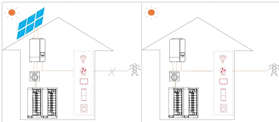
During grid outages, loads can be powered by the battery and PV system.
