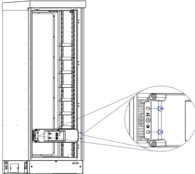
Step 3 Push the HV box into the rack and fasten it with screws
