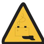
Battery may leak corrosive electrolyte.
