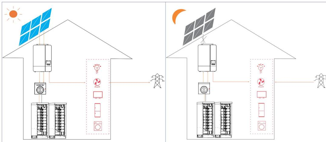
The PV system optimizes energy for loads, and excess energy charges the battery before exporting to the grid.
