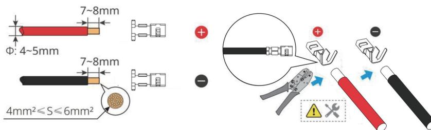
Step 3: Insert the crimp contact into the connector until it audiblysnaps into place. Pull the cable gently backward to ensure a firm connecti
