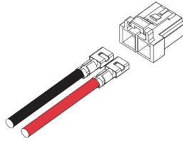
Step 4: Connect the connector to the power terminal of the battery. When you hear a “Click”, it indicates that the connection is complete.
